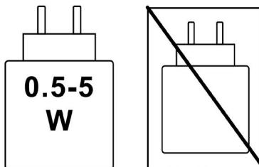
The power supplied by the charger must be between min 0.5 Watts (required by the radio equipment) and a maximum of 5 W to ensure an optimal charging speed.
